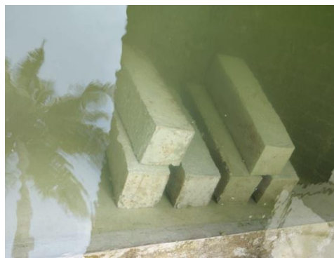
FIG NO.5 NORMAL CURING TANK WITH PRISM
