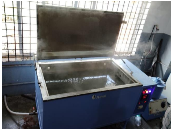
FIG NO.4 STEAM CURING TANK WITH PRISM
