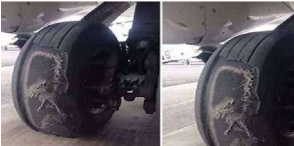
Figure 2: Worn out tyres
