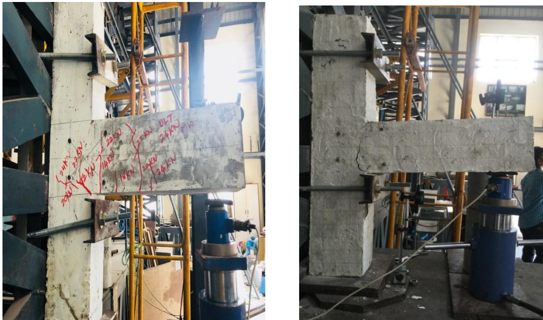
Figure 5 Failure Pattern of Beam-Column Joint
