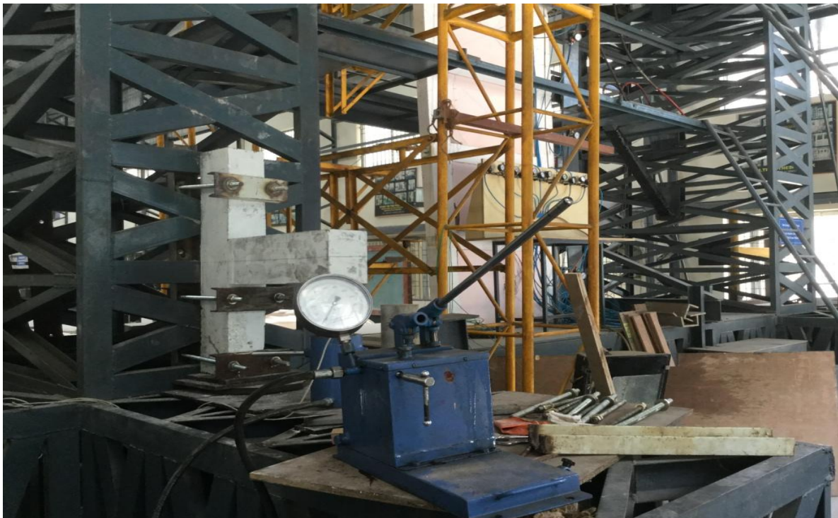
Figure 4 Test Setup of Beam-Column Joint
