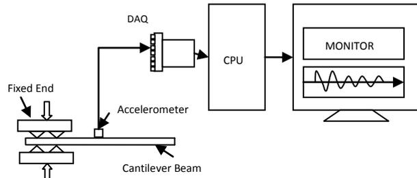
Fig. 2.1 Schematic diagram of vibration measuring apparatus
