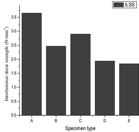
Fig. 3.3 Comparison of Interlaminar shear strengths of Composites
