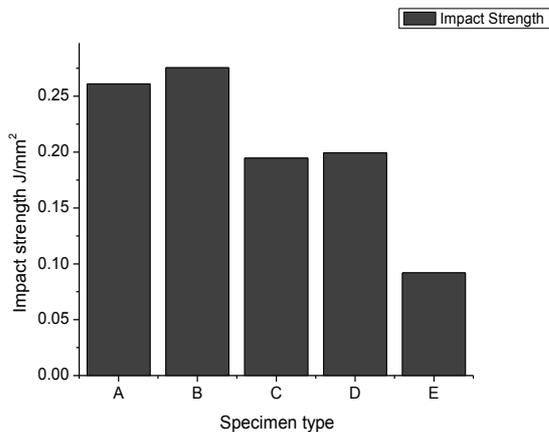
Fig. 3.1 Comparison of impact strengths of Composites
