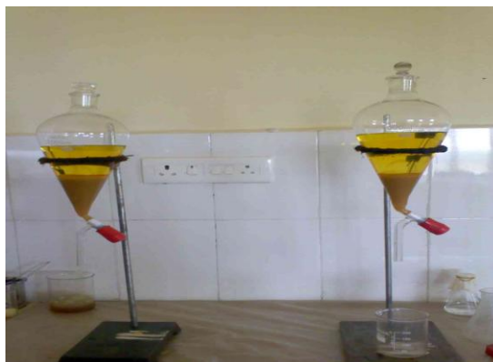
Fig. 7 Separation of Bio Diesel
