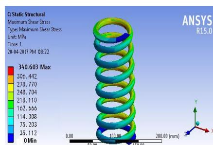
Figure.4: Maximum shear stress for Chrome silicon spring
