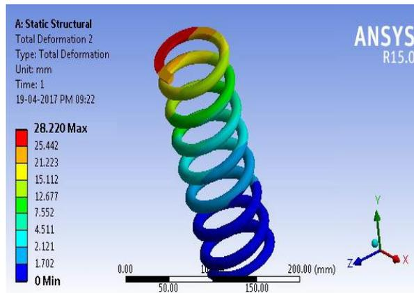
Figure.6: maximum deflection for chromesilicon spring
