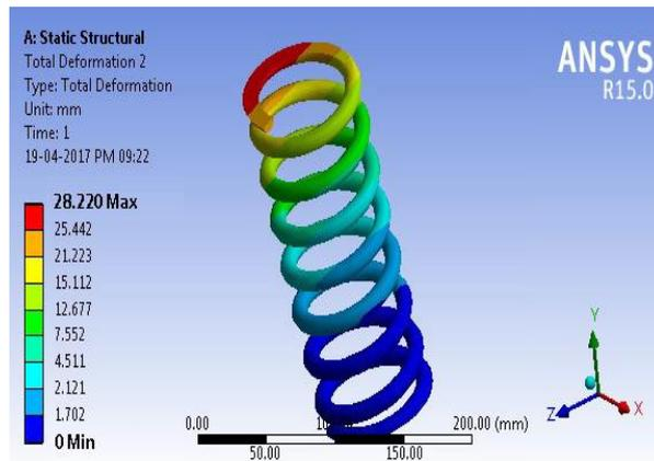
Figure.6: maximum deflection for chromesilicon spring
