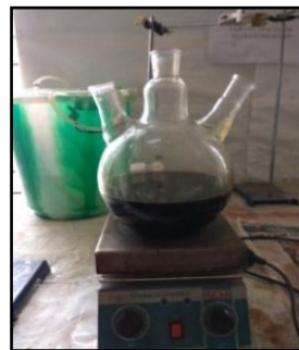
Fig 5: Heating of biodiesel to remove moisture and methanol
