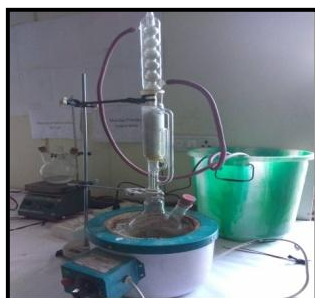
Fig 1: Soxhlet extraction set up
