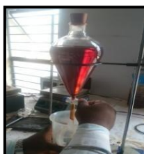
Fig 2: Settling process of FFA
