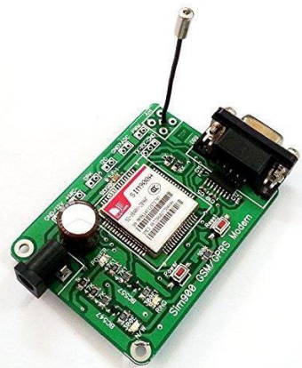
Figure 2 SIM900 GSM/GPRS Module
