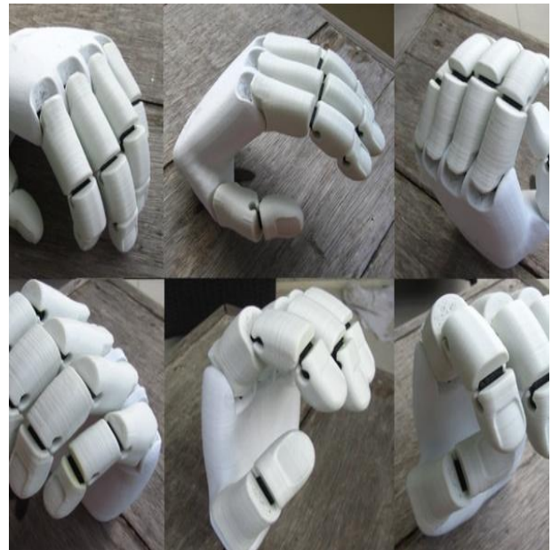
Figure 8: shows various actions performed using the prosthetic arm
