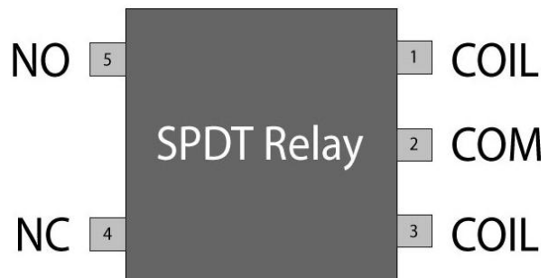
Fig 7. SPDT Pin out diagram
