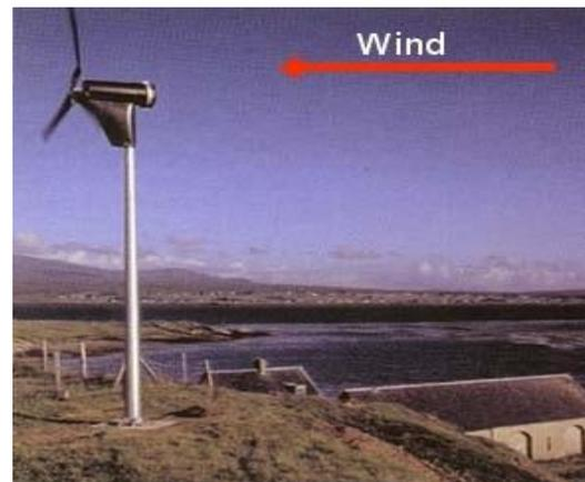
Figure 3 Downwind Mill
