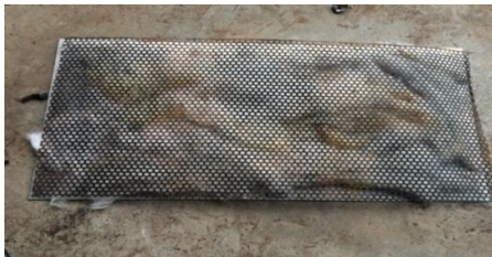
Fig.3 Metallic sheets with glass-wool
