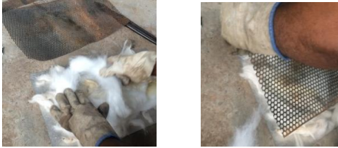
Fig.2 View of metallic sheets of M4 muffler
