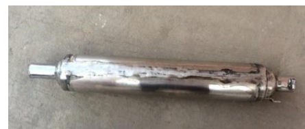
Fig. 9 View of modified muffler (M4)
