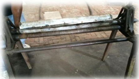
Fig.4 Sheets rolled in bending machine
