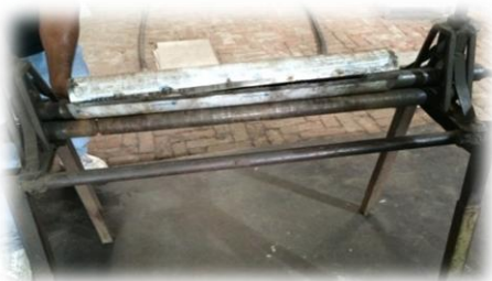
Fig.4 Sheets rolled in bending machine
