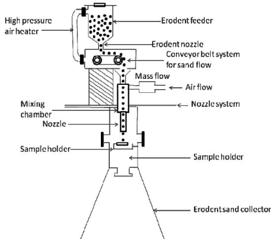
Fig. 1. A schematic diagram of air jet erosion test rig.
