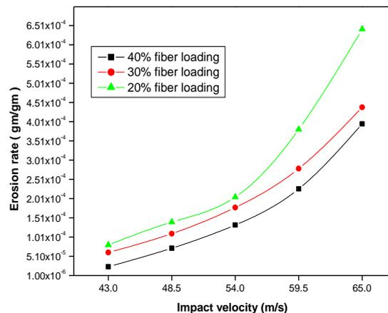
Fig. 3. Variation of erosion wear rate with impact velocity at constant Impingement angle 60 $^\circ$ , Stand of distance 75mm and Erodent size 450 $\mu\text{m}$ .
