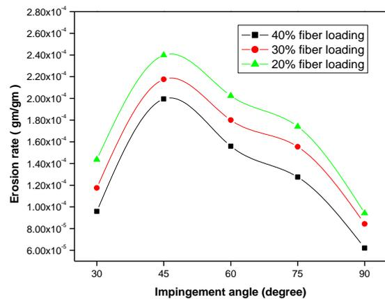
Fig. 2. Variation of erosion rate with impingement angle at constant Impact velocity 45m/s, Stand of distance 75mm and Erodent particle size 450 $\mu\text{m}$ .
