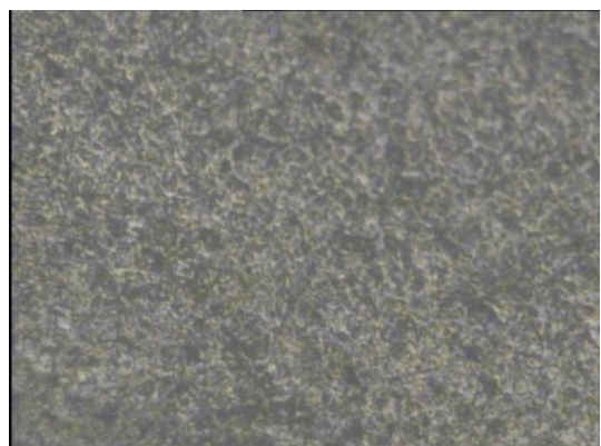
Fig.12. Microstructure of Welded Specimen (6% Cu and rest is 2014 Series Al).
