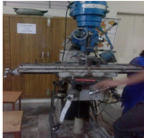
Fig.3. Friction Stir Welding Setup
