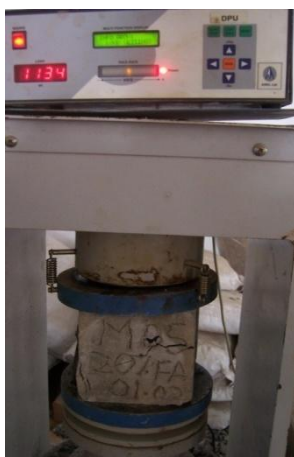
Fig. 4. Compressive strength of cube specimen after failure
