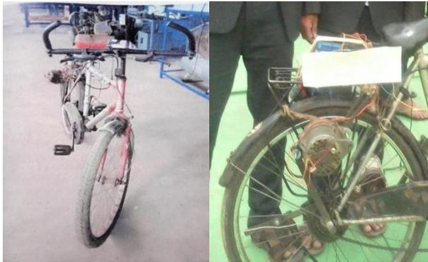
Fig. 1. electromechanical bicycle
