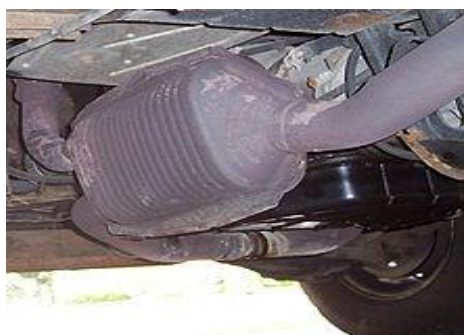
Fig. 16. Three-way catalytic converter on a gasoline - powdered.
