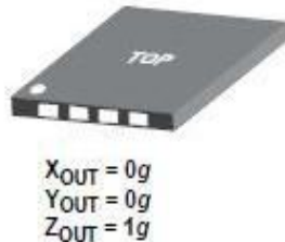
Fig 6.1 Values of Z= 1g position for measuring
