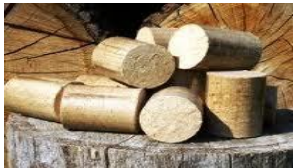
Fig. 2. Samples briquettes produced with 100% waste
