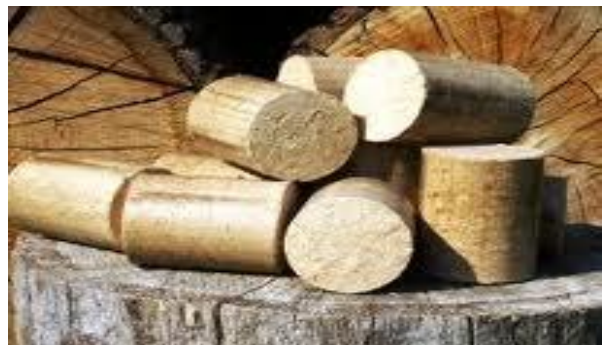
Fig. 2. Samples briquettes produced with 100% waste
