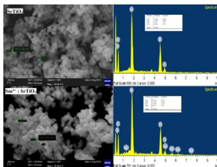
Fig.3 SEM & EDS images of the SrTiO<sub>3</sub> & Sm<sup>3+</sup>:SrTiO<sub>3</sub> ceramic powders
