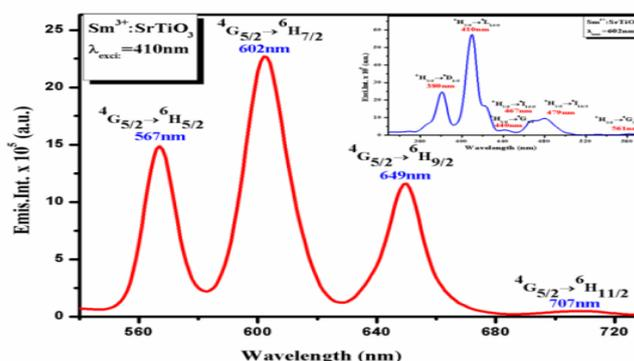
Fig. 4 Emission spectrum ( $\lambda_{\text{exc}} = 410\text{nm}$ ) of Sm<sup>3+</sup>:SrTiO<sub>3</sub> ceramic powder (inset figure: Excitation spectrum ( $\lambda_{\text{emi}} = 602\text{nm}$ ))
