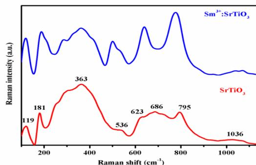
Fig.2 Raman spectrum of  $\text{SrTiO}_3$  &  $\text{Sm}^{3+}:\text{SrTiO}_3$  ceramic powders
