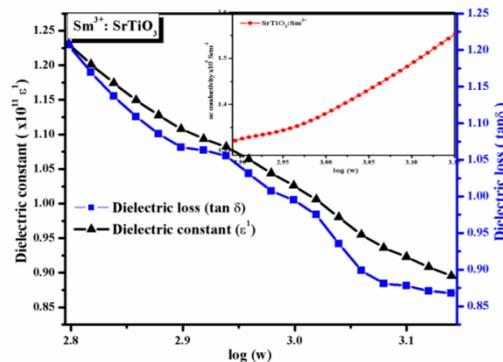
Fig.8 Dielectric constant ( $\epsilon'$ ), loss factor ( $\tan\delta$ ) & ac conductivity (inset figure) of  $\text{Sm}^{3+}$ :  $\text{SrTiO}_3$  ceramic powder
