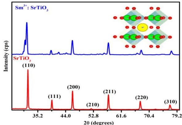
Fig.1 XRD profile of  $\text{SrTiO}_3$  &  $\text{Sm}^{3+}:\text{SrTiO}_3$  ceramic powders (inset figure shows perovskite  $\text{SrTiO}_3$ )
