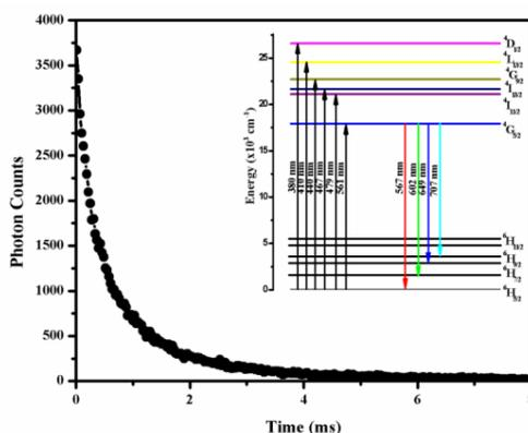
Fig.5 Decay curve of  $\text{Sm}^{3+}:\text{SrTiO}_3$  ceramic powder (inset figure shows an energy level diagram of the  $\text{Sm}^{3+}:\text{SrTiO}_3$  ceramic powder)
