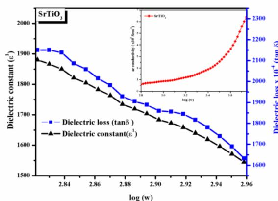
Fig.7 Dielectric constant ( $\epsilon'$ ), loss factor ( $\tan\delta$ ) & ac conductivity (inset figure) of  $\text{SrTiO}_3$  ceramic powder
