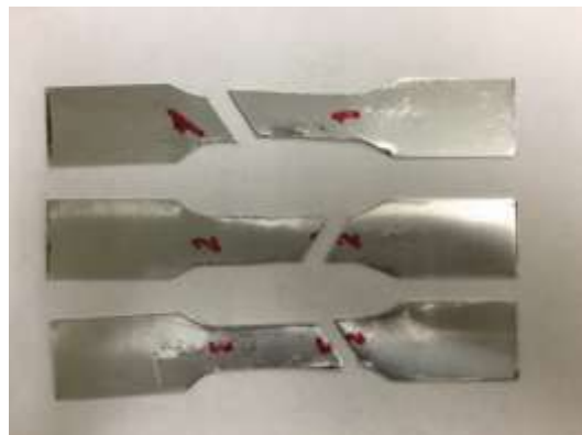
Fig. 1 Aspects of Aluminum Specimens after Tensile Test
