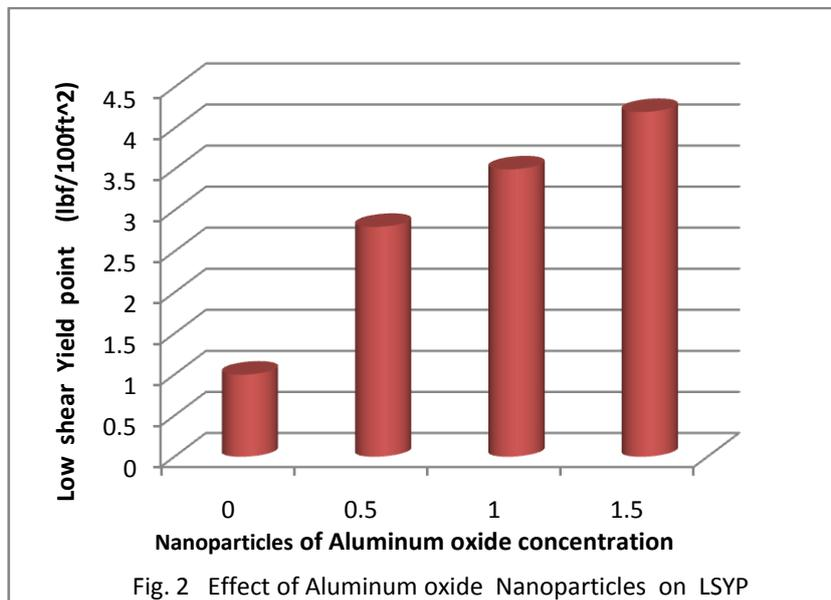
Fig. 2 Effect of Aluminum oxide Nanoparticles on LSYP
