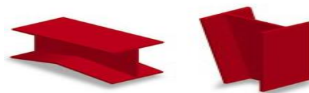
Fig.1.1 Built-Up "I" Shaped Primary Structural Framing Members.
