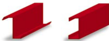
Fig.1.2 Cold-Formed "Z" And "C" Structural Members.
