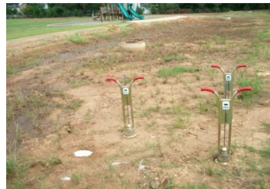
Fig. 4. Photographs showing the infiltration measurement setups at the Shelby Park biofilter
