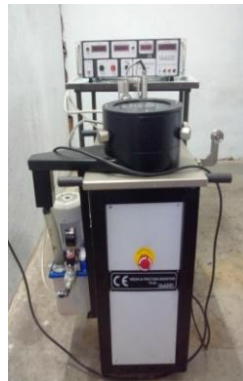
Fig.2.1 Pin-on-disc wear testing machine Microstructure figures
