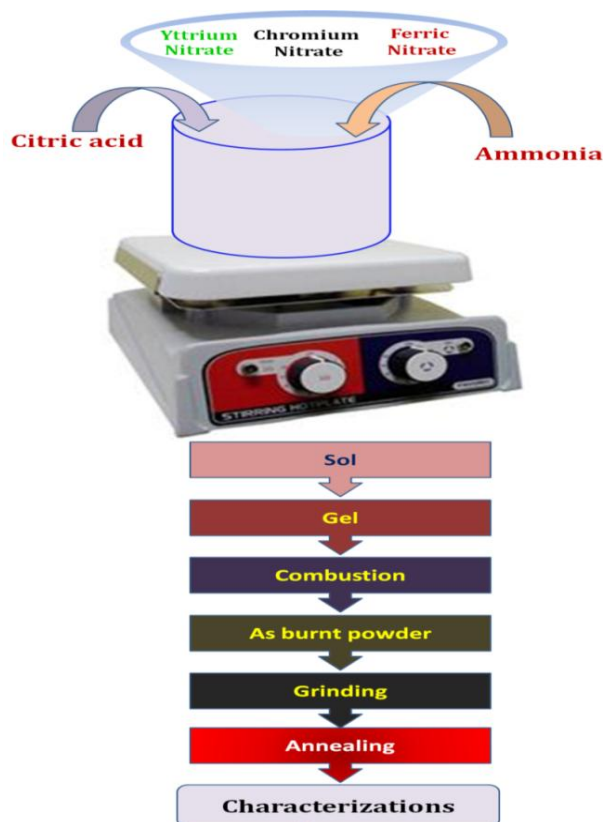
Fig. 1. Schematic flowchart of sol-gel auto combustion synthesis route for preparation of Y_3Fe_{5-x}Cr_xO_{12}
