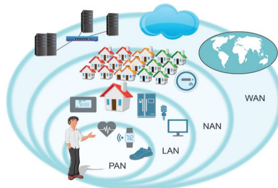
Fig 2. Different ranges and applications for personal, local, neighborhood and wide area networks
