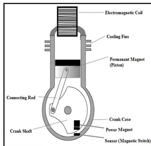
3.1 Concept diagram of single cylinder electromagnetic engine
