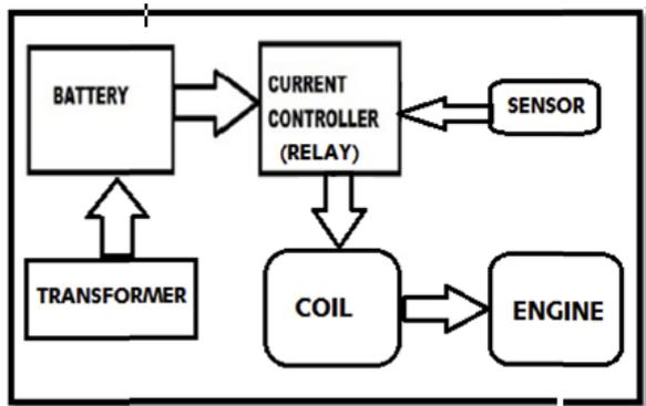
**5.1 Block Diagram of proposed engine**
