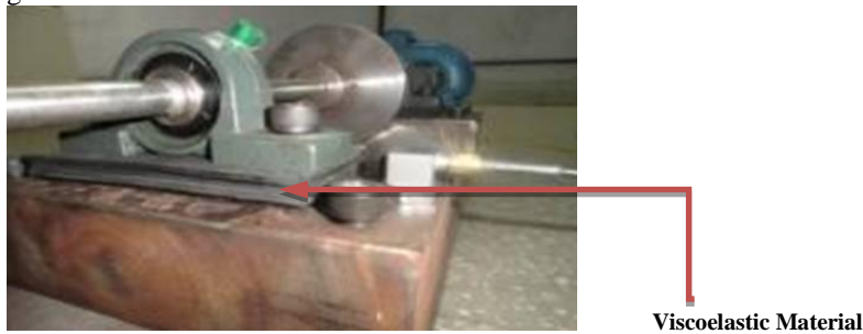
Fig.6:Arrangement of Viscoelastic support beneath bearing housing for different cases
