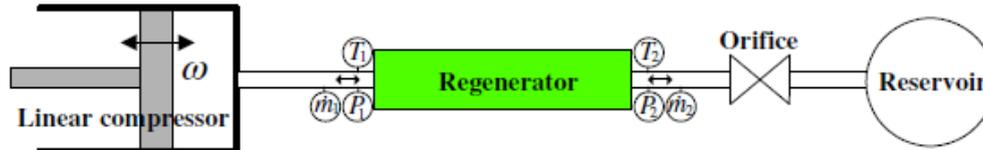
Fig 1: Schematic diagram of experimental apparatus
