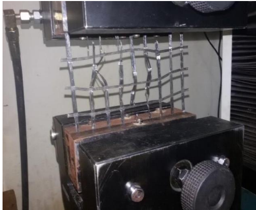
Fig. 1 Tensile testing of geogrid
