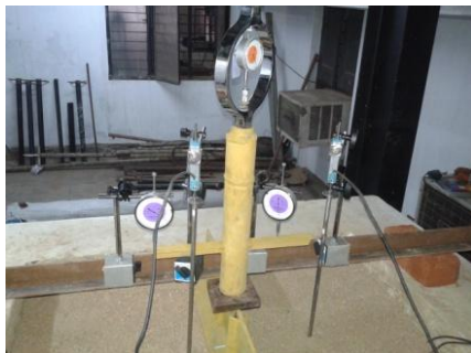
Fig. 8. Arrangement for application of load and Measurement of settlement
