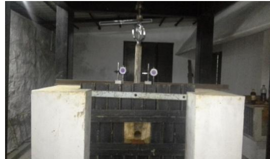
Fig. 7. Void in Soil after removing pipe
