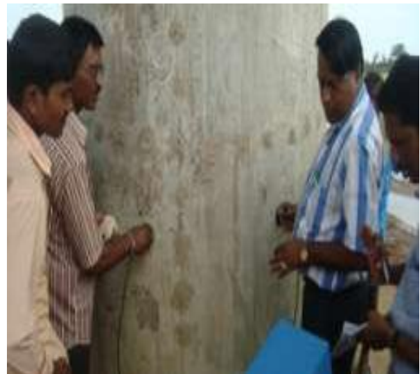
Fig 9: Testing of Bridge Pier using Ultrasonic Tester
