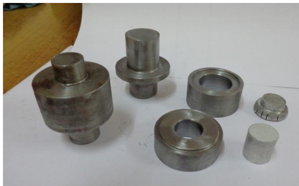
Figure 2 Die set to fabricate circular-head rivet form sintered porous specimen
