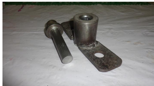
Figure 1 Die set used to fabricate cylindrical porous composite specimen
