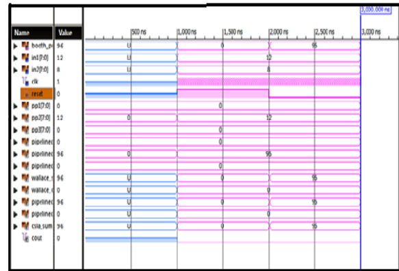
Figure 5 Simulation result for modified boothencoded multiplier
