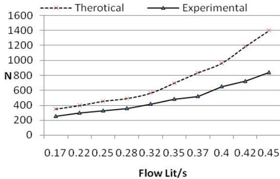
Fig. 5b: A plot of Flow v/s Speed for 6 smooth discs and 0.55mm spacing
