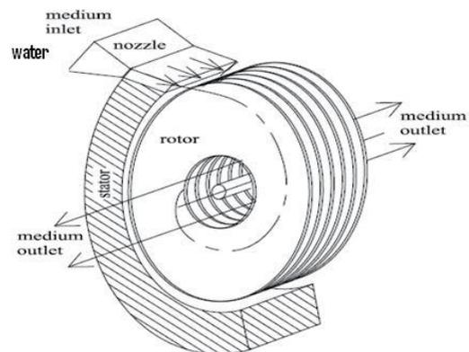
Fig. 3: Cross Section of Test Rig
