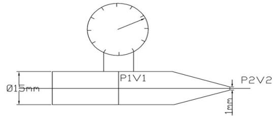
Fig. 1: Nozzle Arrangement – line diagram for Test Rig By applying Bernoulli's equation, at point1 and at point2
