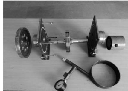
Fig. 2: Parts of Multiple disc Turbine.
