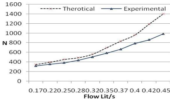
Fig. 6: A plot of Flow v/s speed for 6 Rough discs and 1.4mm spacing
