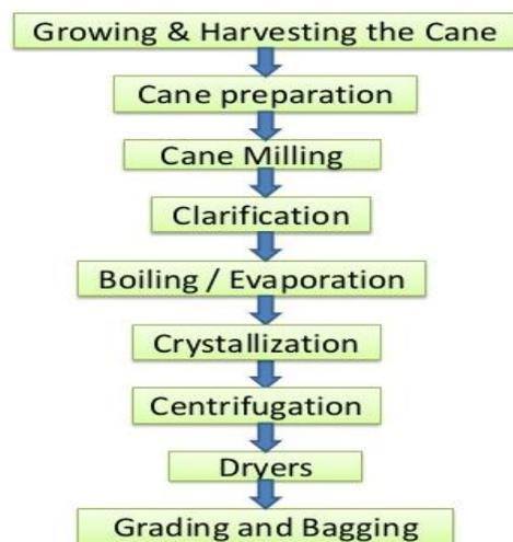
Fig 1: sugar manufacturing process flow chart
