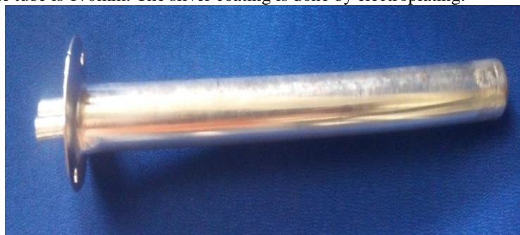
Figure 2 Silver Coated Condenser
