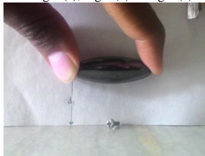
Fig. 4(a) The distance between nail & magnet from where magnet starts attracting/pulling small nail ( d_1 )
