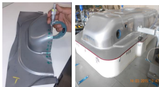
Fig 11 (a) Thinning measurements using point micrometer, (b)Component check on gauge
