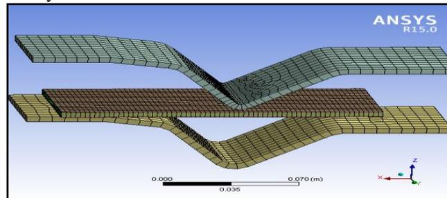
Fig 2.2 Map Meshed Geometry
