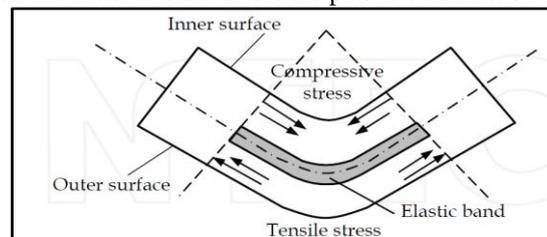
Fig. 1.2. Illustration of the Elastic Band in the Bend part
