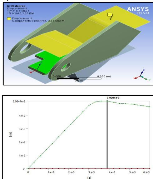
Fig.3.4 Displacement of component
