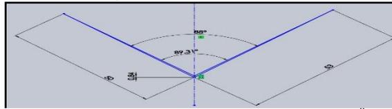
Fig.3.9 spring back when die valley angle 88<sup>0</sup>
