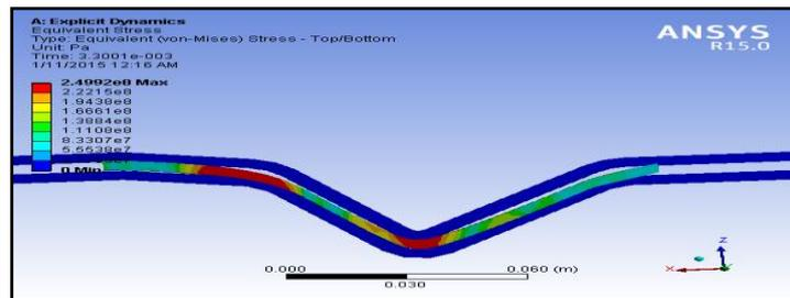
Fig 3.7 Final Vonmises stress during loading
