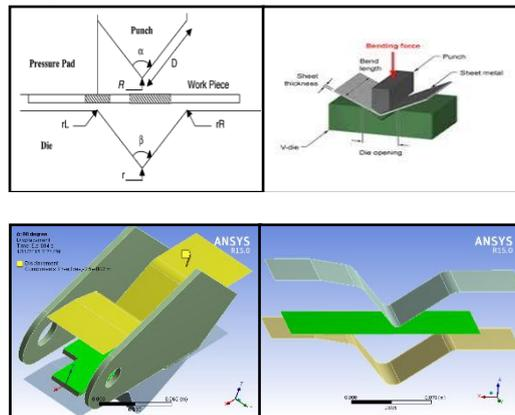
Fig.2.1 FEA Model set-up
