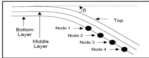
Fig.3.6 spring back calculation
