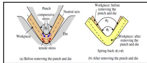
Fig. 1.1 Spring Back Principle
