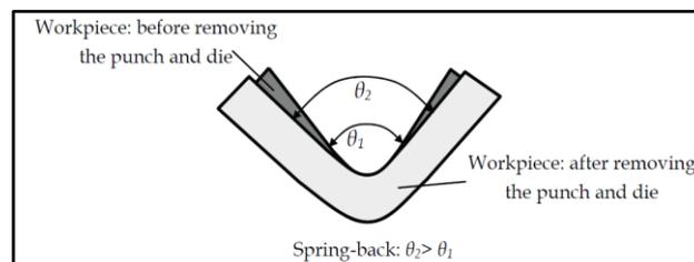
Fig. 1.3. Illustration of Spring-back Feature
