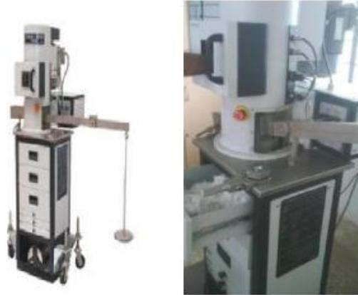
Fig.1 Four Ball Tester
