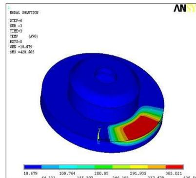
At t = 3.0 sec,  $T_{\max} = 428.563 \text{ } ^\circ\text{C}$
