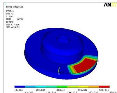
At t = 2.0 sec,  $T_{\max} = 428.95 \text{ } ^\circ\text{C}$
