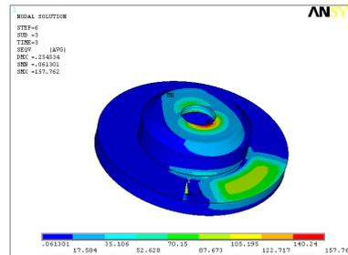
Fig. 5.11 Von Mises stress contour plot for C.I. Solid disc
