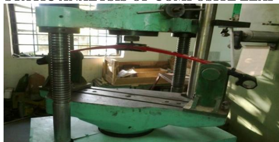
Fig.1 Static Analysis of Composite Leaf Spring
