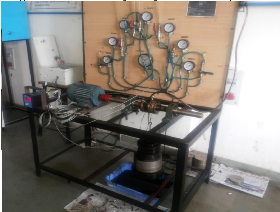
Fig. 3 Journal Bearing Test Rig
