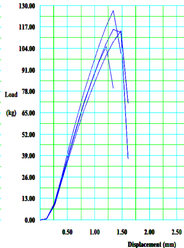
Fig.1 Tensile Characteristics of WS-PP composite Fig.2 Tensile Characteristics of J-PP composite
