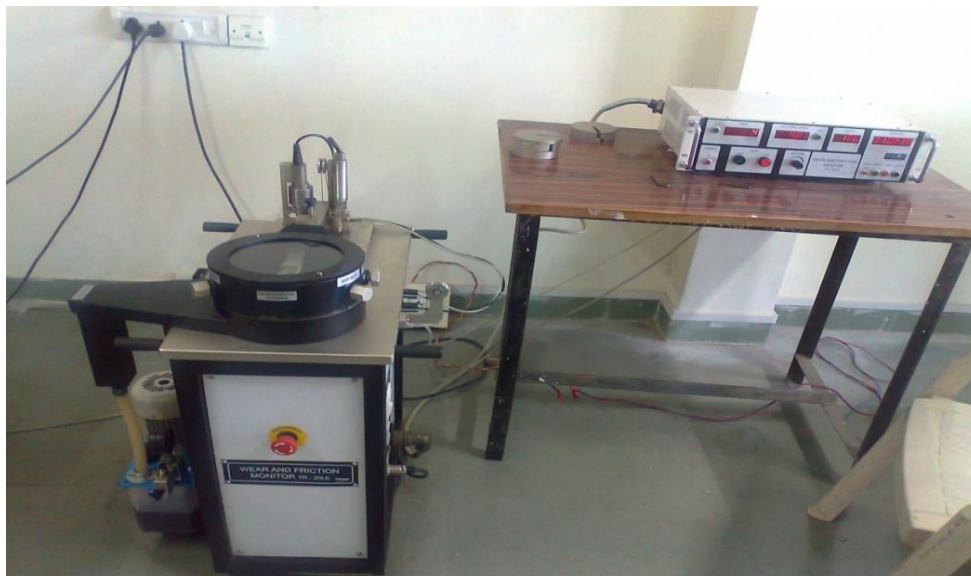
Fig1 Photograph of Experimental Set up (Tribometer TR-20LE )
