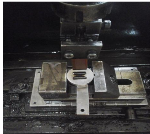
Fig 1: Machining of concave profile on Monel 400 by EDM
