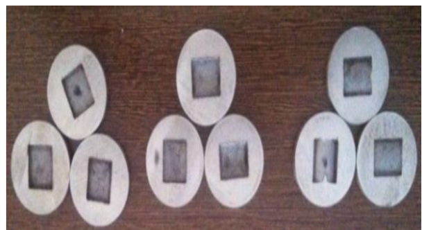
Fig 2: Flat, Concave and convex profile on Monel 400 by EDM
