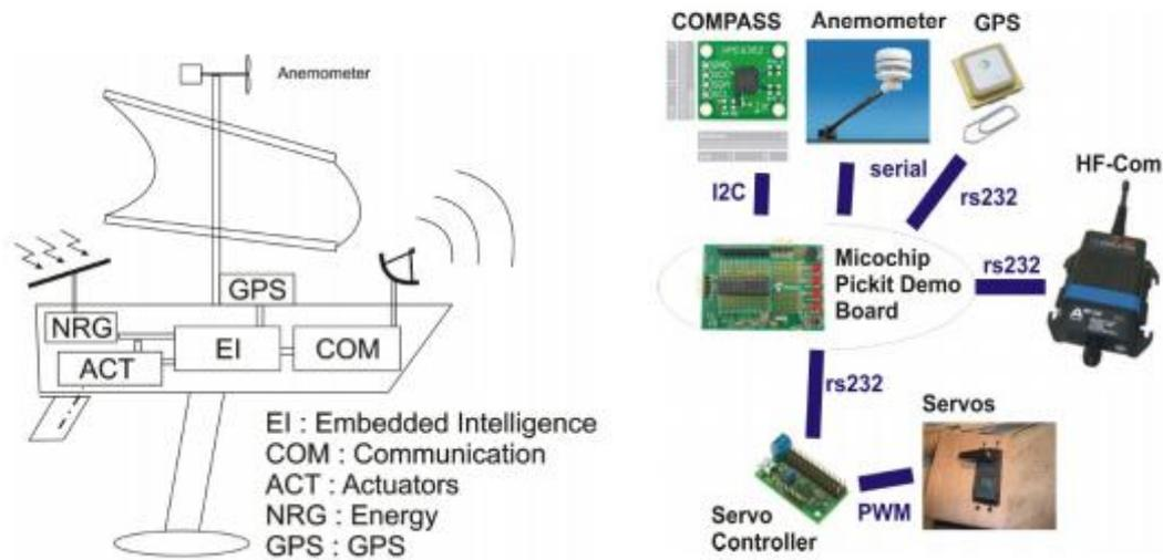
Fig. 1 Hardware Architecture
