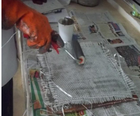
Fig 2 Fabrication by hand lay-up method
