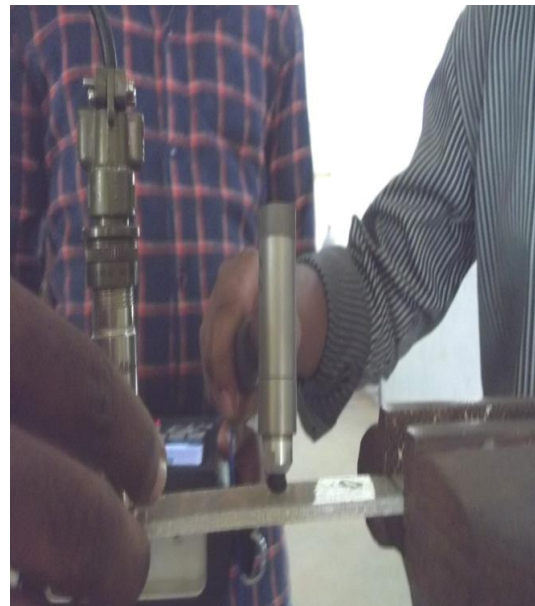
Fig 9 Impact hammer test procedure
