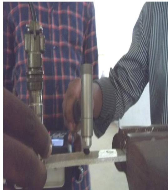
Fig 9 Impact hammer test procedure
